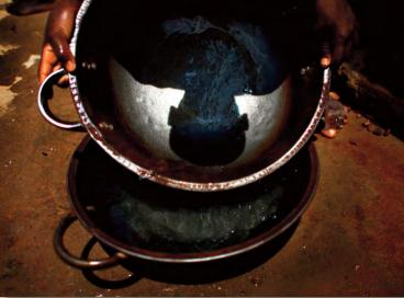
To extract gold from the raw ore, workers must first crush the ore, then wash and strain it through car floor mats. Finally the slurry is ground together by hand with a silvery glob of mercury in large metal wash basins, like the one used here at a gold processing site in Dareta, Nigeria.
